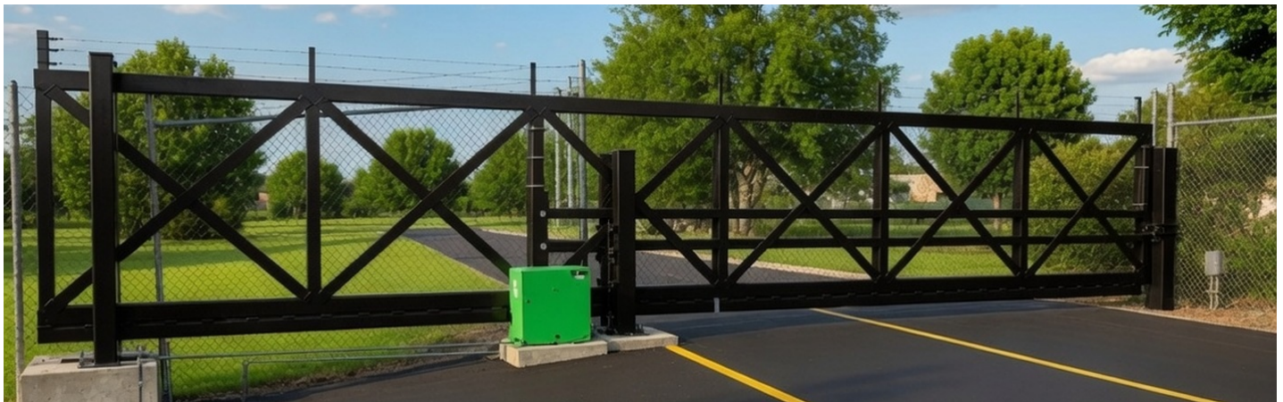
Crash-rated slide gate with a trussed frame and integral operator, on an asphalt drive.
