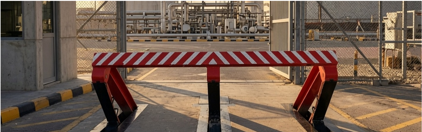
M50 wedge deployed at an energy site entrance. The drive acts directly on the wedge.
