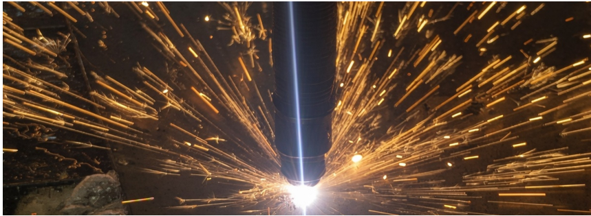
Profile cutting at BSP. SecurePale™ components are cut, formed, galvanized and coated in the United States.
