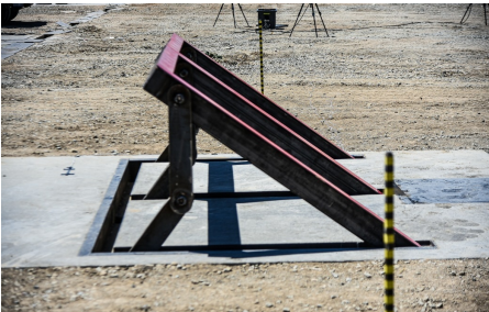
Test article, deployed — 39° of blocking height.
