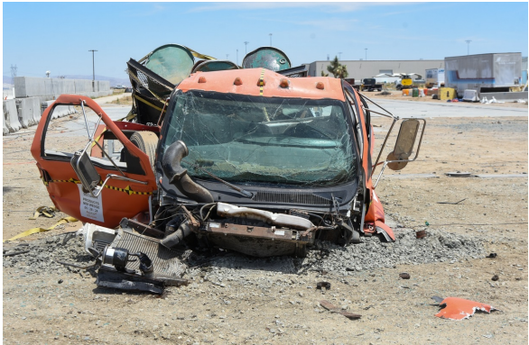
After impact at Applus IDIADA KARCO — the cab has separated from the chassis.
