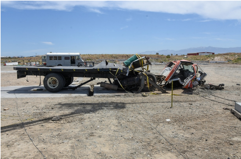
After impact — the cab has been torn from the chassis and the bed has continued past it. The barrier is in the foreground, still seated.
