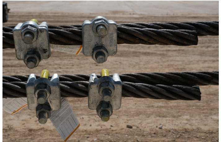
Cables marked and tagged at the posts for crash testing — photographed after the M50 impact at TTI.
