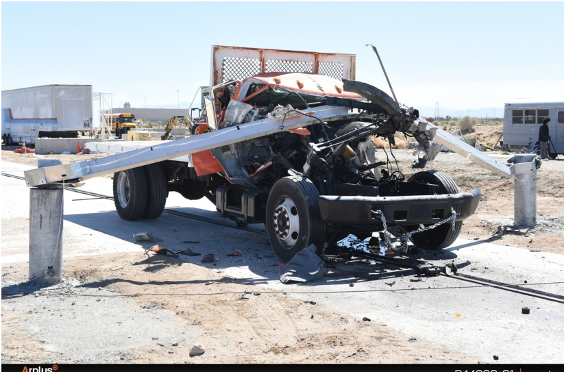
After impact at Applus IDIADA KARCO — the cab is destroyed, the arm is still spanning the opening and both posts are standing.
