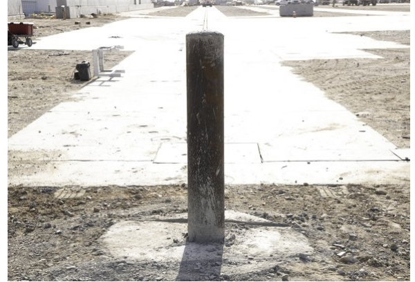
The as-tested article on the tow road at Applus IDIADA — an 8-inch Schedule 40 pipe standing 48 inches above grade, with nothing below it but concrete.
