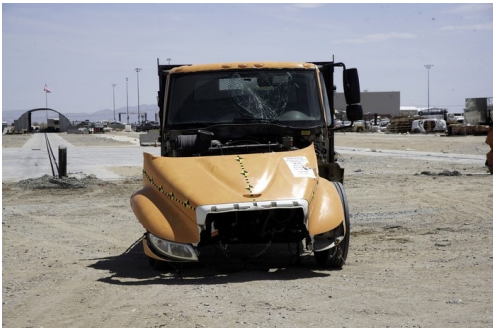
The test vehicle after impact — engine displaced into the cab, disabled where it stopped.
