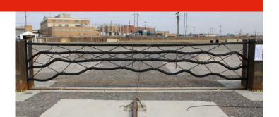
BSP Defender Net Barrier was created to lessen the damage to an accidental impact while maintaining the security of the Anti-Ram vehicle barrier requirements of the KI 2 and M50 certifications. This system has been fully tested and certified to DOD and ASTM requirements to stop a 15,000 lbs. vehicle traveling at 50 mph. Designed as one of the few final denial barriers that utilizes the net based vehicle barrier concept, our net has quickly reached the forefront in the industry.
